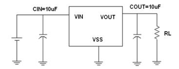
**Suggesting:** The circuit uses the electrolytic capacitors or tantalum capacitors in the best ,when it is applied in the high input voltage.
